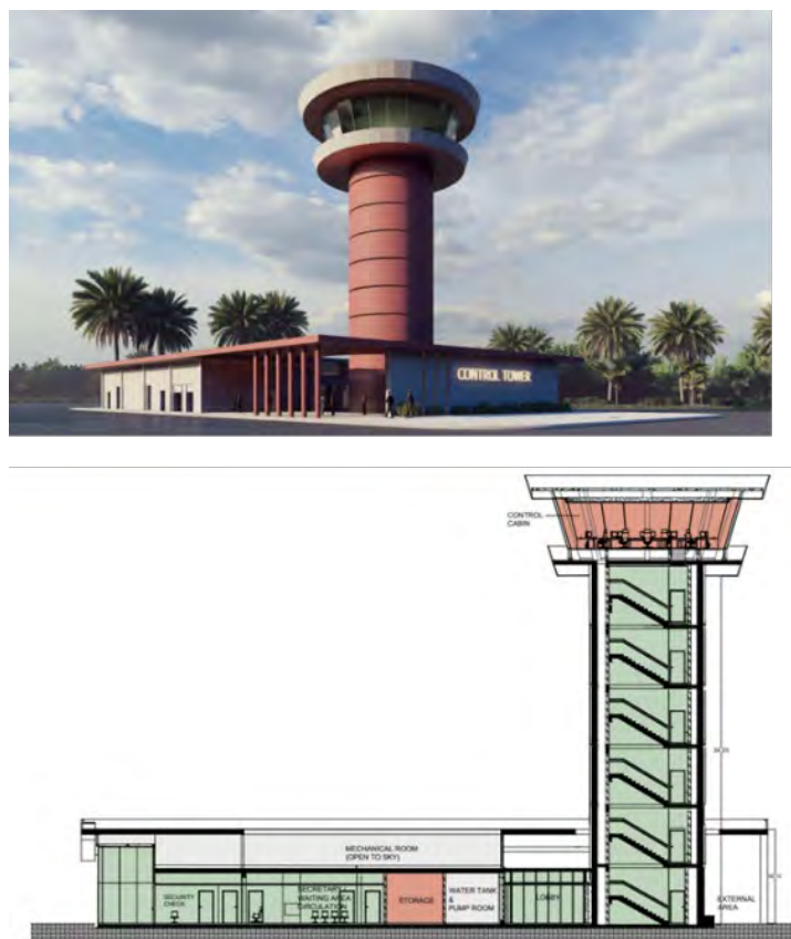
Figure 12: Perspective view of the Control Tower building and section.
